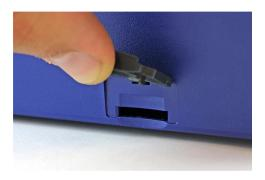
2. Insert the MicroSD\* card into the socket.
