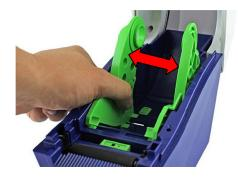
4. Place the roll between the holders and close them onto the core.
