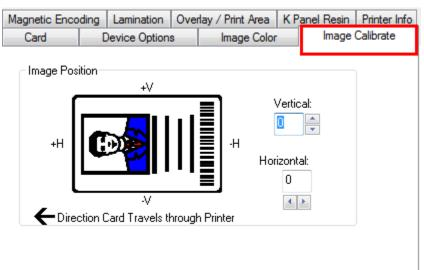
Use the **Vertical** and **Horizontal** image position controls to adjust the position of the overall print area to be precisely centered on a card. The maximum value for the **Vertical** and Horizontal adjustments is ±100 pixels (10 pixels = about .03%, .8mm).
